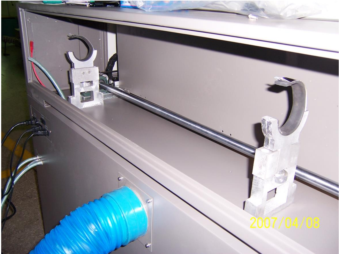
Put the laser tube on two bases.
